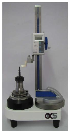
Based on the established alfa-test concentricity testing device
