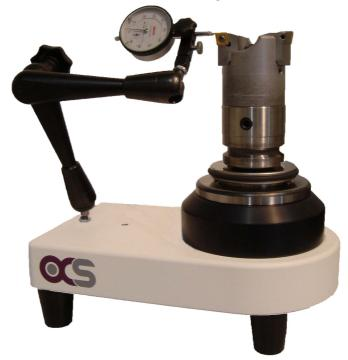
Setting and testing device for rotary cutting tools such as:
